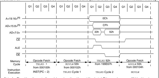
Note 1: The address lines actually used depends on the address width selected. This example assumes 20-bit addressing.
