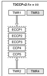
Timer1 is used for all Capture and Compare operations for all CCP modules. Timer2 is used for PWM operations for all CCP modules. Modules may share either timer resource as a common time base.
