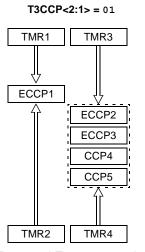
Timer1 and Timer2 are used for Capture and Compare or PWM operations for ECCP1 only (depending on selected mode).
