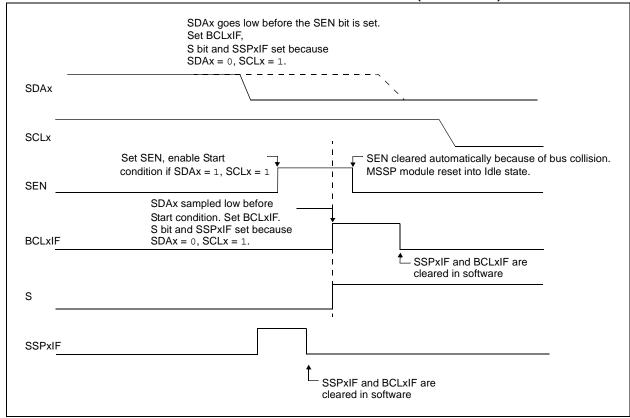
FIGURE 19-27: BUS COLLISION DURING START CONDITION (SCLx = 0)
