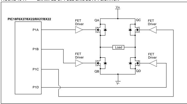
FIGURE 18-7: EXAMPLE OF FULL-BRIDGE APPLICATION
