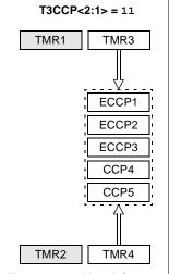
Timer3 is used for all Capture and Compare operations for all CCP modules. Timer4 is used for PWM operations for all CCP modules. Modules may share either timer resource as a common time base.
