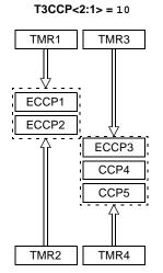
Timer1 and Timer2 are used for Capture and Compare or PWM operations for ECCP1 and ECCP2 only (depending on the mode selected for each module). Both modules may use a timer as a common time base if they are both in Capture/Compare or PWM modes.
