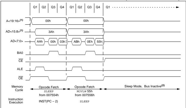
Note 1: The address lines actually used depends on the address width selected. This example assumes 20-bit addressing.
