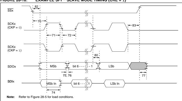
FIGURE 28-18: EXAMPLE SPI™ SLAVE MODE TIMING (CKE = 1)
