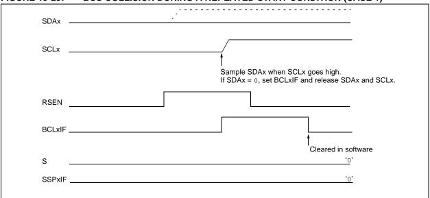
FIGURE 19-30: BUS COLLISION DURING REPEATED START CONDITION (CASE 2)
