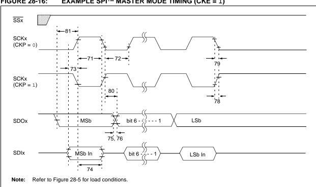
FIGURE 28-16: **EXAMPLE SPI™ MASTER MODE TIMING (CKE = 1)**
