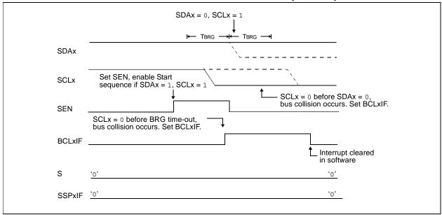
FIGURE 19-28: BRG RESET DUE TO SDAX ARBITRATION DURING START CONDITION
