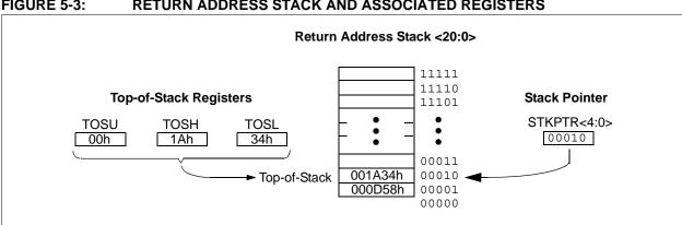
FIGURE 5-3: RETURN ADDRESS STACK AND ASSOCIATED REGISTERS
