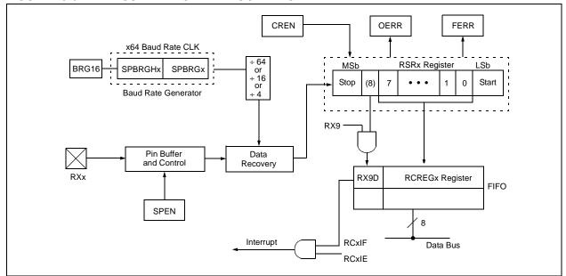
FIGURE 20-7: ASYNCHRONOUS RECEPTION
