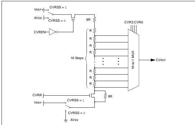
FIGURE 23-1: COMPARATOR VOLTAGE REFERENCE BLOCK DIAGRAM
