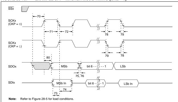
FIGURE 28-15: EXAMPLE SPI™ MASTER MODE TIMING (CKE = 0)
