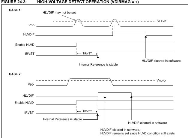
**FIGURE 24-3: HIGH-VOLTAGE DETECT OPERATION (VDIRMAG = 1)**
