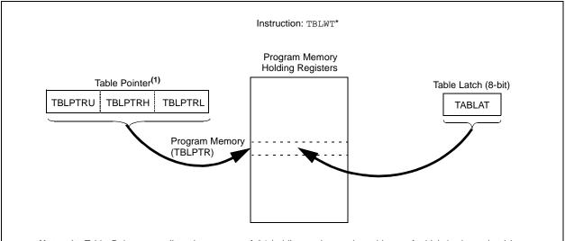
Note 1: Table Pointer actually points to one of 64 holding registers, the address of which is determined by TBLPTRL<5:0>. The process for physically writing data to the program memory array is discussed in Section 6.5 "Writing to Flash Program Memory".
