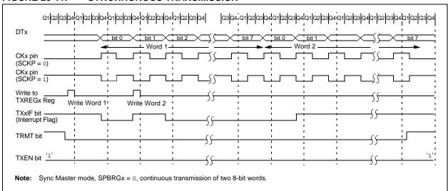
FIGURE 20-12: SYNCHRONOUS TRANSMISSION (THROUGH TXEN)
