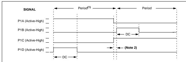
Note 1: The direction bit in the ECCP1 Control register (CCP1CON<7>) is written any time during the PWM cycle.
