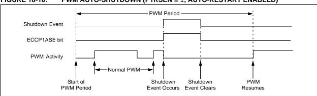
FIGURE 18-10: PWM AUTO-SHUTDOWN (P1RSEN = 1, AUTO-RESTART ENABLED)
