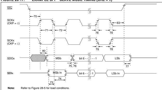
FIGURE 28-17: EXAMPLE SPI™ SLAVE MODE TIMING (CKE = 0)
