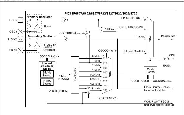
FIGURE 2-11: PIC18F8722 FAMILY CLOCK DIAGRAM
