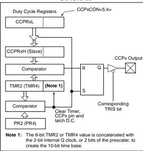
A PWM output (Figure 17-5) has a time base (period) and a time that the output stays high (duty cycle). The frequency of the PWM is the inverse of the period (1/period).
