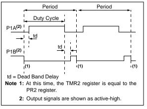
FIGURE 18-5: EXAMPLES OF HALF-BRIDGE OUTPUT MODE APPLICATIONS
