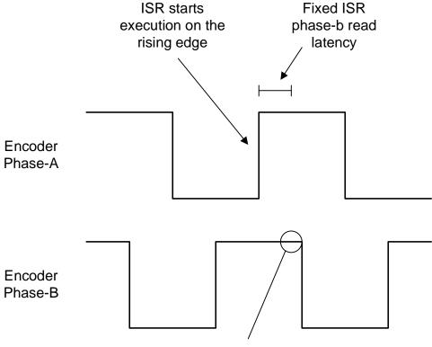
Under normal circumstances, the ISR will read the state of phase-b and correctly determine the direction the shaft is rotating
